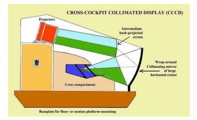
Digital imaging improved more or less in parallel with increases in computing power and continues to improve. These advances have lead to the production of so-called wrap around visuals in flight simulators and has transformed the industry. With such a visual, it is possible to fly a "visual" circuit around a runway observing the landing area in the correct sense from all points in the circuit.
