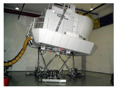
However the simulation of acceleration in flight simulators remains limited and, in fighter aircraft whose accelerations are typically large and sustained, motion simulation is not used.
