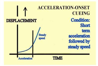
As the jacks reach the limit of travel, the rate of displacement is reduced to zero at a rate which is below the threshold of human sensory system, the so-called washout phase.
